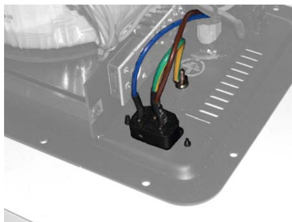
Figure 5. The IEC connector, as mounted to the HPR amplifier module chassis. Note the wire colors and the terminals they connect to; the new connector must be wired exactly the same way.
